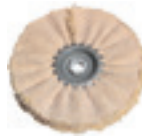
FELT LAMELLA ROLLER For polishing and pre-polishing stainless steel. Because of the lamella, the felt doesn't "burn" and polishing without streaks is possible. Only use with polishing paste (pre-polishing = pre-polishing paste, high-gloss polishing = colouring paste).
