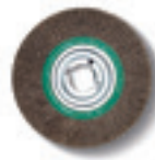
STEEL WIRE BRUSH Ø 250 mm x 60 mm, with very high wire drawing strength for highly efficient use, mounting hole Ø 51 mm. 0.2 mm thick wire for thin-walled pipes and profiles. 0.35 mm-thick wire for universal use. 0.5 mm thick wire for thick-walled pipes and profiles and great deburring results. Stainless steel version
