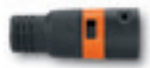
ANTISTATIC TOOL COLLAR Electrically conducting, with suction force regulation, for hose diameter 35 mm, power tool connection (diameter 27 mm).
