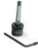
3/4" WELDON MOUNTING SHAFT for using FEIN core drills on bench and column drilling machines and all other core drilling units with MT fitting. With internal cooling lubricant supply. Tool-free core drill bit changes.
