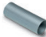
HOSE Flexible, for swarf extraction, 90 mm in diameter, 1 m long, steel, high level of heat resistance.
