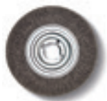
STEEL WIRE BRUSH Ø 250 mm x 60 mm, with very high wire drawing strength for highly efficient use, mounting hole Ø 51 mm. 0.2 mm thick wire for thin-walled pipes and profiles. 0.35 mm-thick wire for universal use. 0.5 mm thick wire for thick-walled pipes and profiles and great deburring results. Steel version
